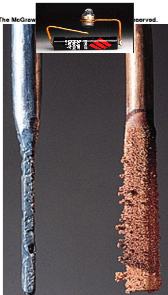
Zinc-Copper Reaction Voltaic Cell
