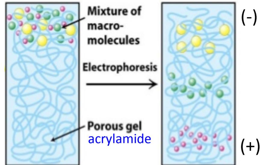
After mixed with Laemmli buffer all proteins are linear and negatively charged therefore proteins separated by size
