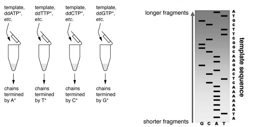
run products in four separate lanes on gel, expose X-ray film "one pot" sequencing more common today:
